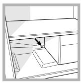
by the compressor causes it to evaporate. It is necessary to clean the discharge hole regularly so that the water can flow out easily.
